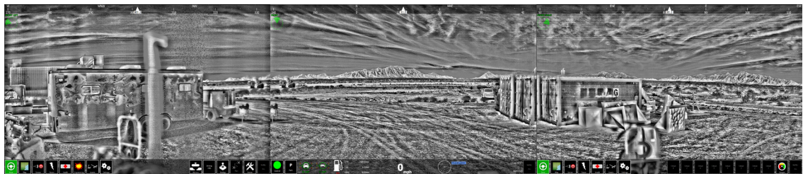
Figure 7.11: IE driving aid in clear environment with dust algorithm.
