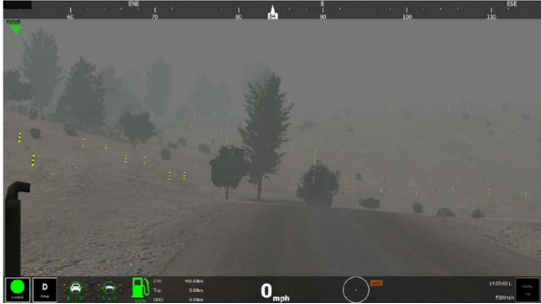
Figure 5.4: Go/NoGo driving aid showing boundary markers in moderate DVE.
