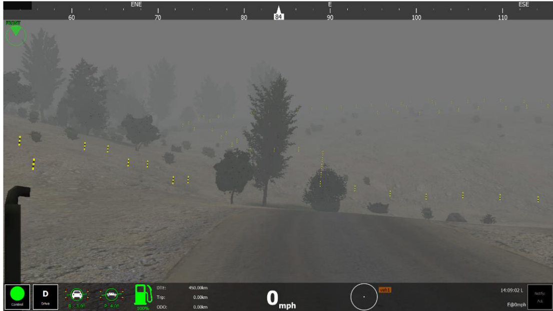
Figure 1.6: Go/NoGo Driving Aid showing terrain slope
