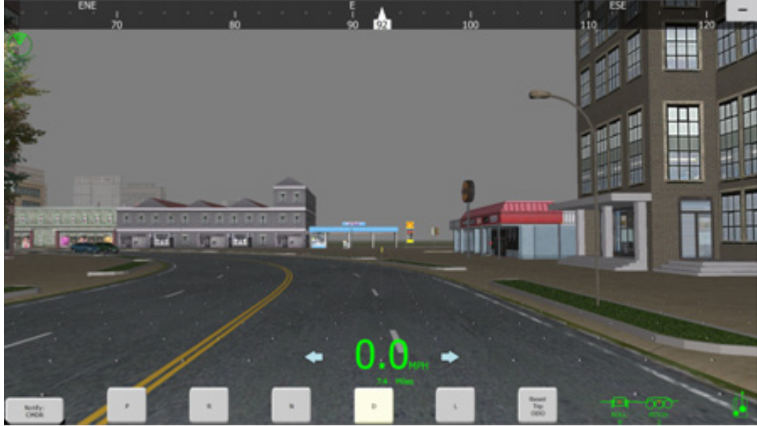
Figure 3.4: Urban route with Optic Flow Driving aid presented as dots at ground level
