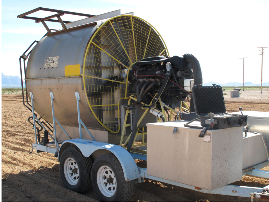
Figure 7.3: Blown Air Dust and Sand System (BADSS).
