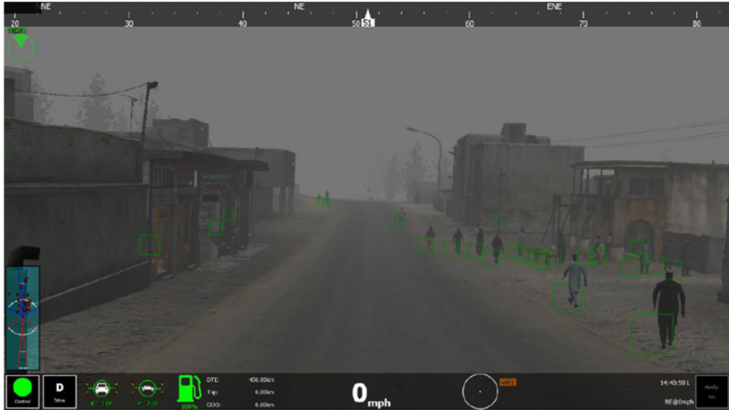
Figure 5.3: Radar driving aid highlighting obstacles with moderate DVE.
